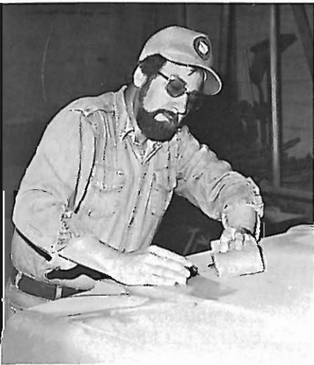
John Gray, Body Repairman and Painter with 7 years service, sand the hood of a truck for finish work.
