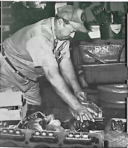
Kenny Wright, Senior Mechanic, 5 years service, overhauls a diesel engine in the district headquarters shop.
